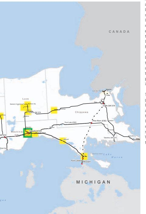
Areas in the western and far eastern Upper Peninsula are most vulnerable to low voltages. The most notable areas experiencing transmission service limitations include the Plains-Stiles 138-kV line and the Hiawatha-Indian Lake 69-kV line. Both of these lines are being addressed for the near term with projects planned for completion in 2006.
