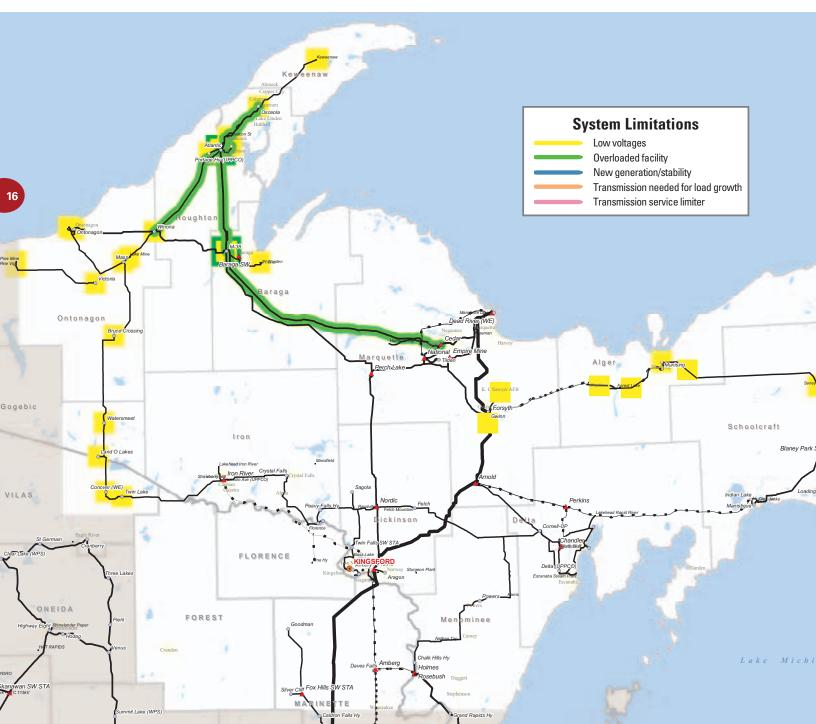
There are a number of transmission system performance issues in Zone 2 including limited ability to import or export power, generator instability, voltage instability, overloaded lines and equipment, low system voltages and chronic limitations to transmission service. Primary drivers of these issues include a mismatch of low-cost generation to load in the Upper Peninsula and aging facilities in poor or obsolete condition.
